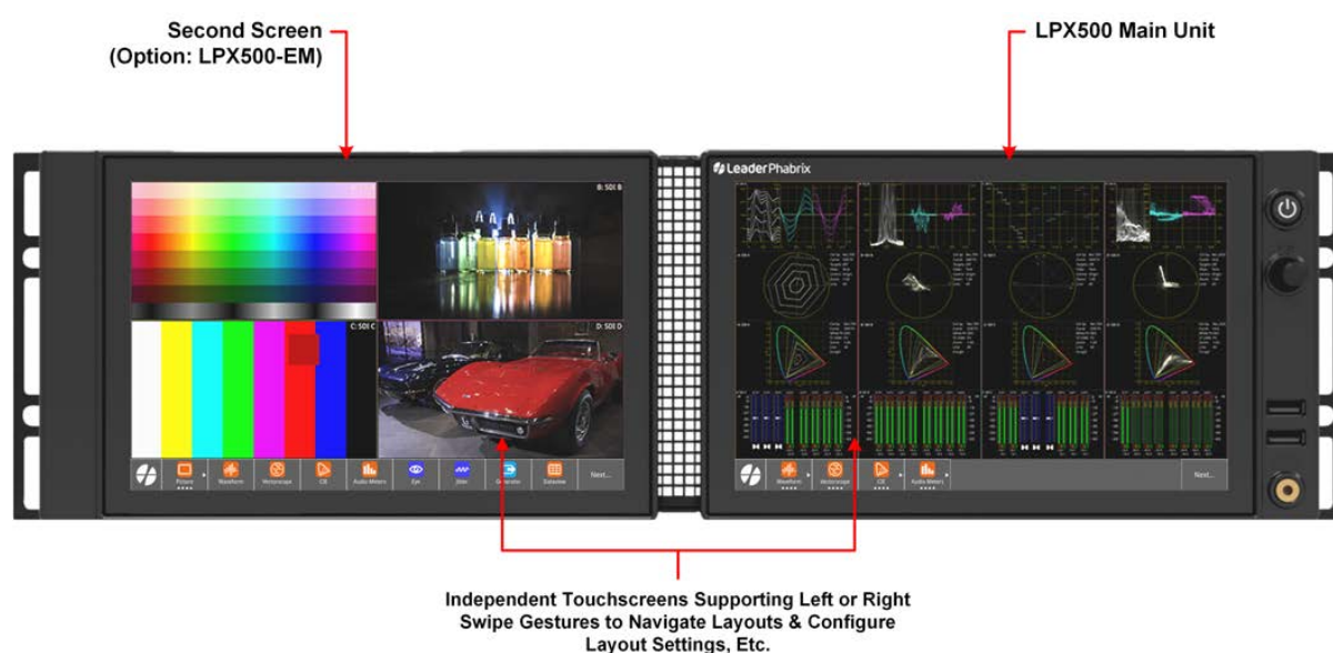
Figure 2-95: LPX500 with Optional Second Screen Connected (Shown in the Rack Mount)
