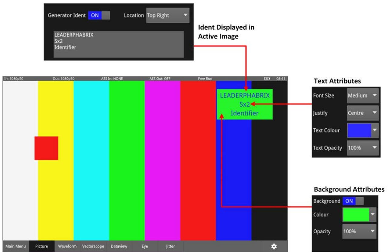
Figure 3-11: Generator Ident Displayed in Picture Display
