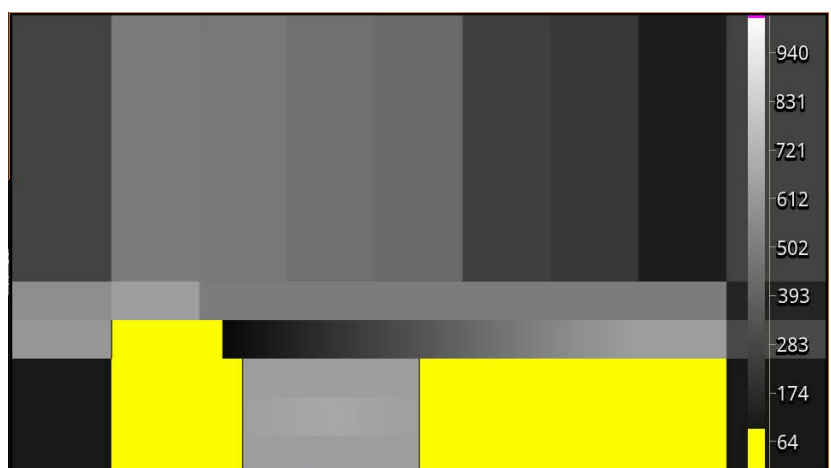
Figure 4-12: False Color Overlay Scale Applied (Decimal Luminance Scale)
