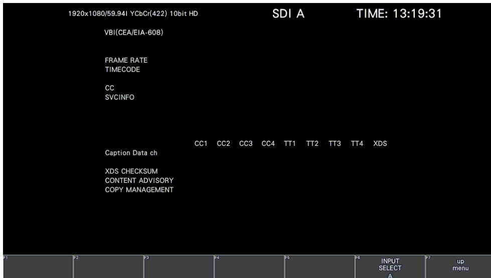
Figure 16-58 VBI data display
