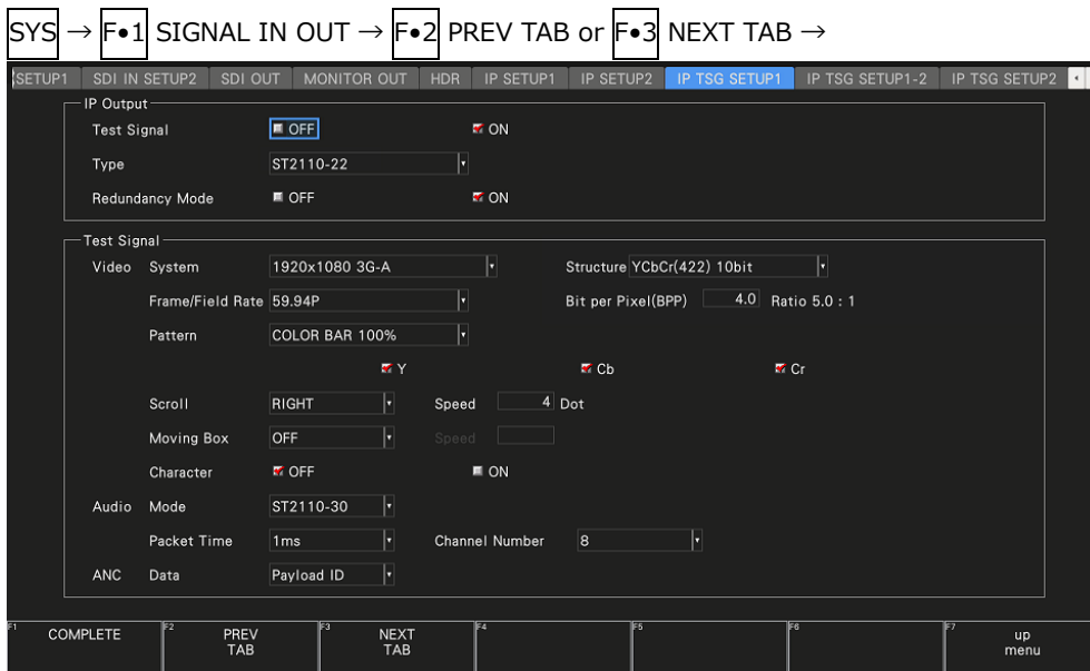
Figure 7-18 IP TSG SETUP1 tab
