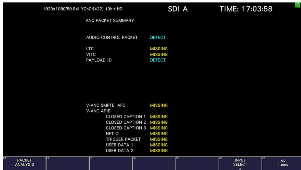
Figure 16-43 Ancillary packet screen
