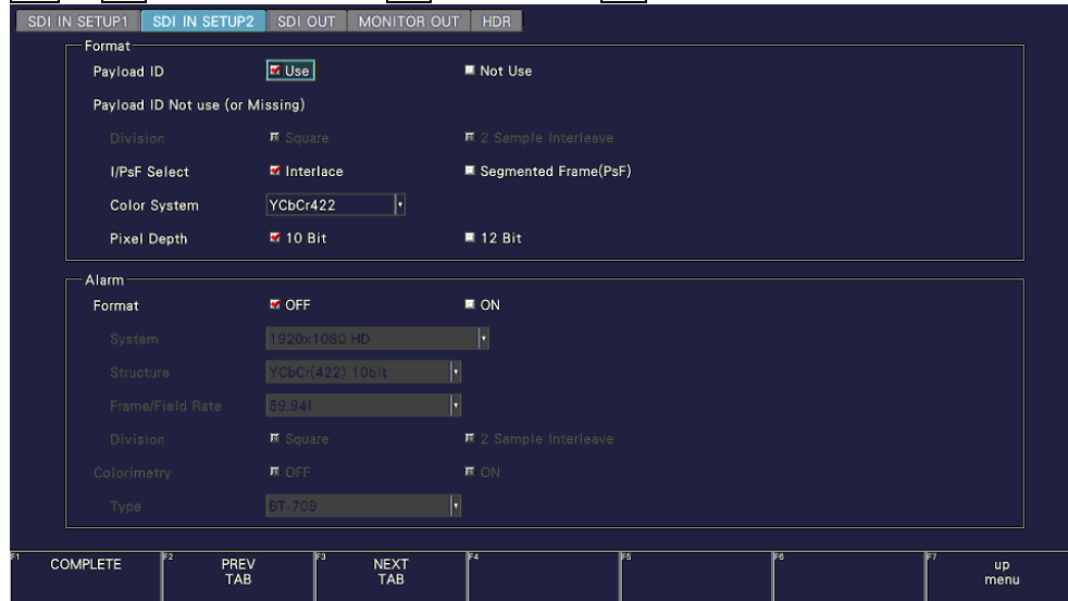
Figure 6-4 SDI IN SETUP2 tab
