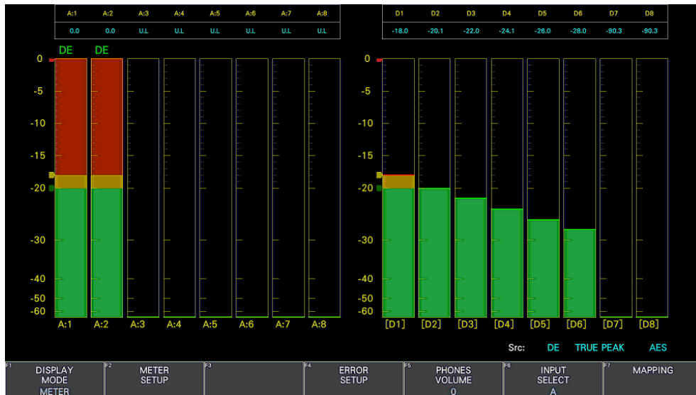
Figure 15-6 AES Dolby display (mix)
