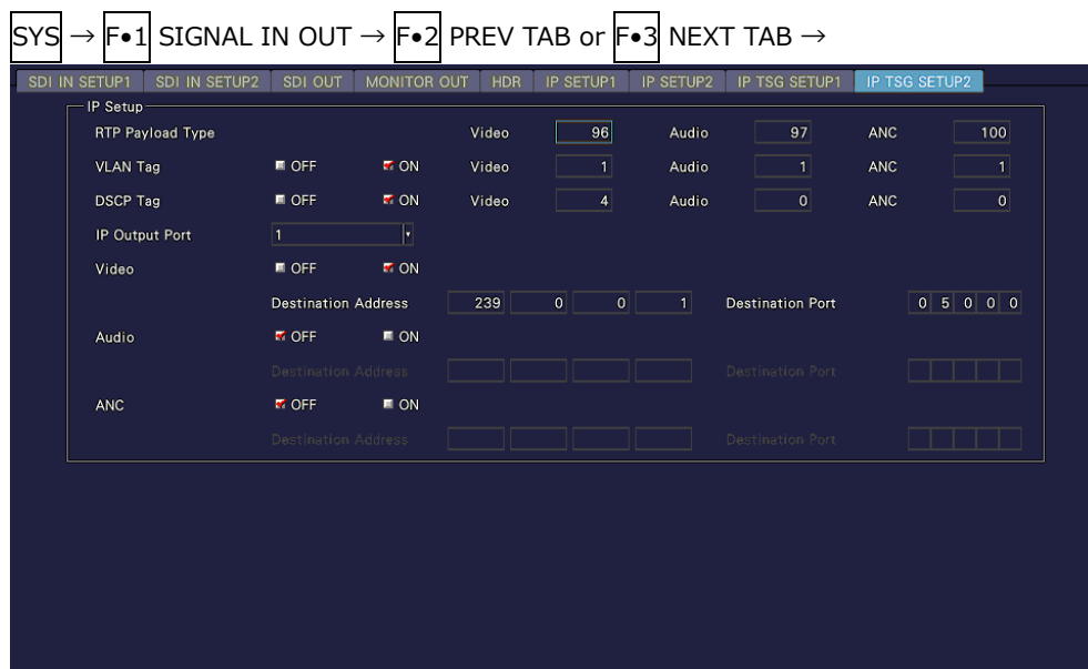
Figure 7-21 IP TSG SETUP2 tab
