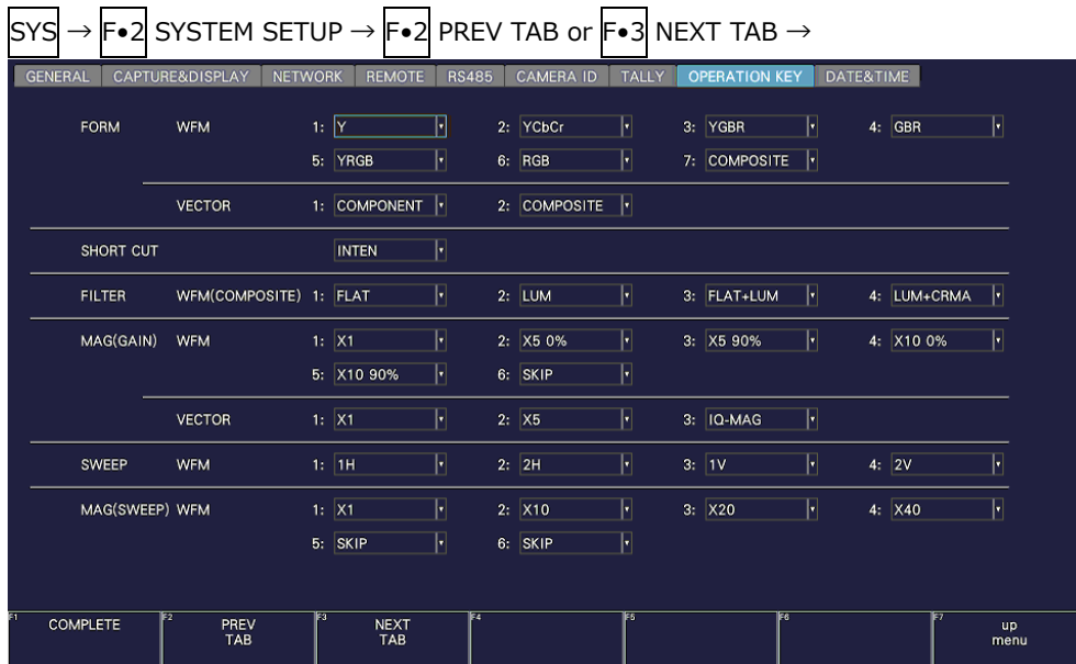
Figure 7-44 OPERATION KEY tab
