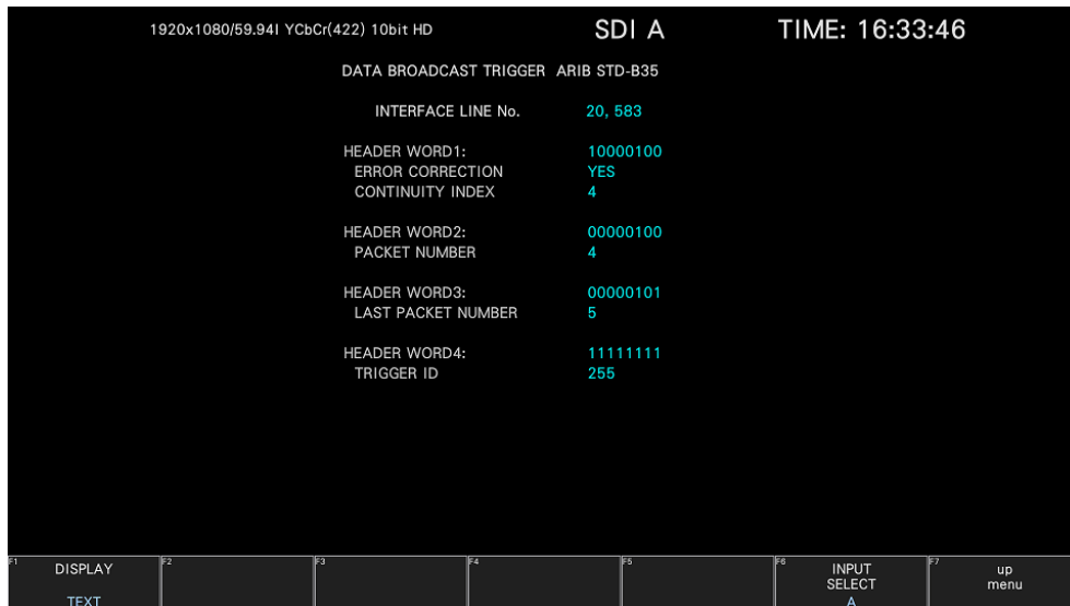
Figure 16-52 Data broadcast trigger signal screen
