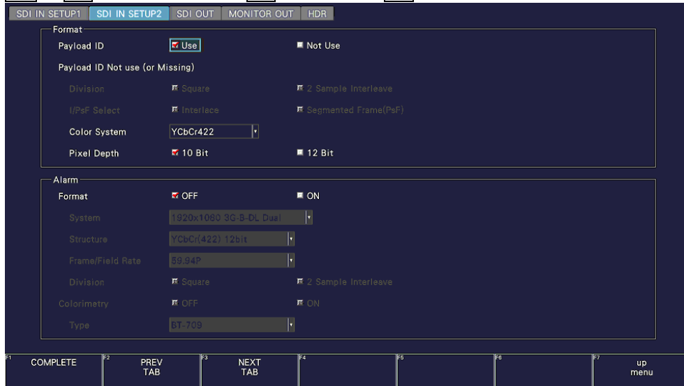
Figure 6-12 SDI IN SETUP2 tab
