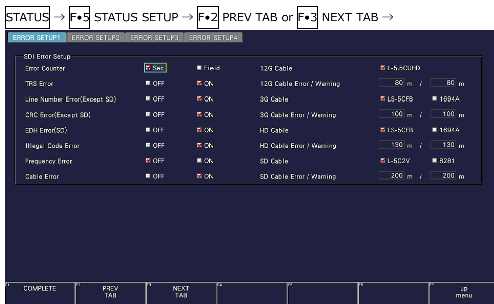
Figure 16-2 ERROR SETUP1 tab
