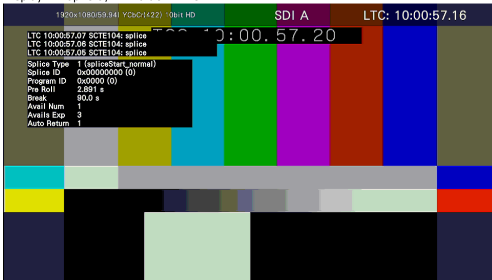
Figure 13-11 SCTE-104 Detection screen
