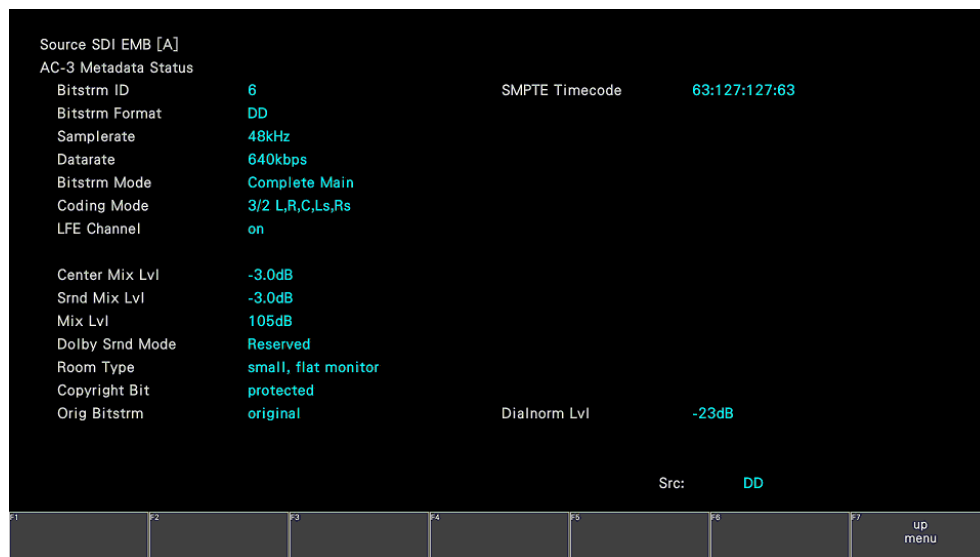
Figure 15-30 Dolby Digital metadata display
