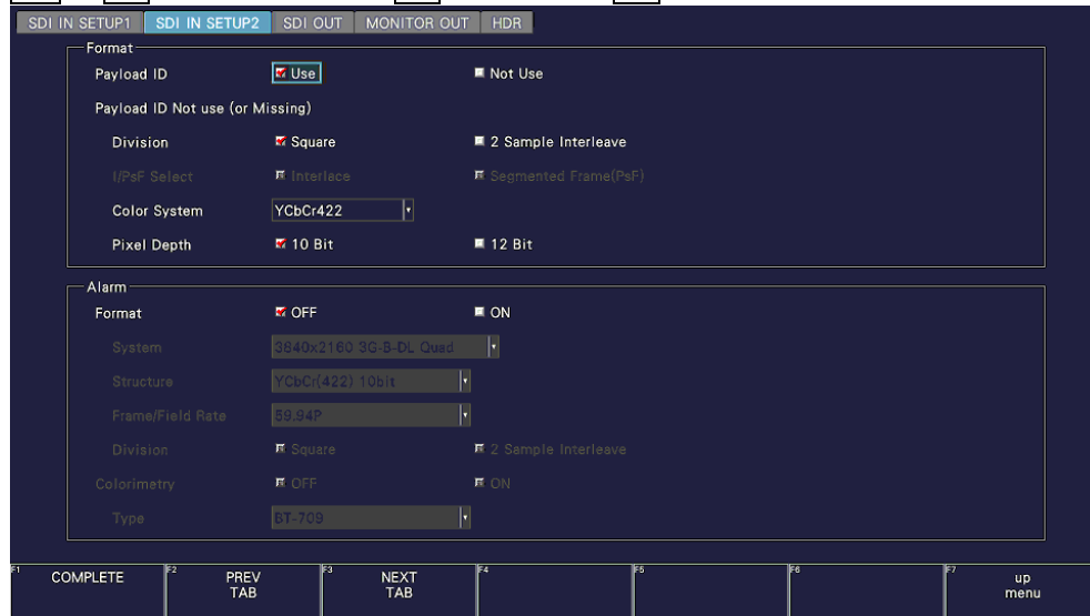
Figure 6-28 SDI IN SETUP2 tab
