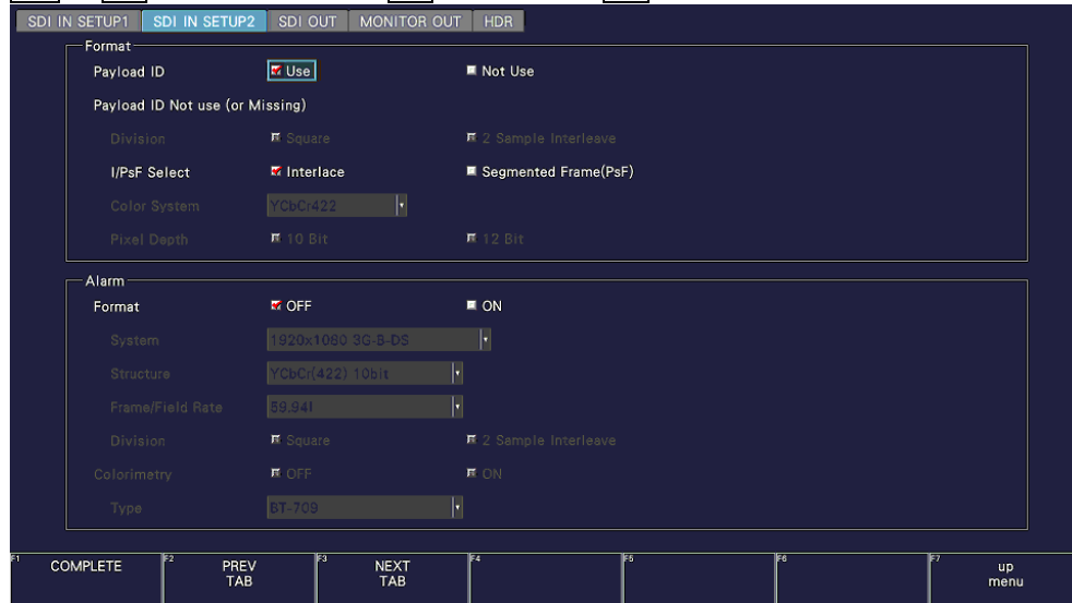
Figure 6-16 SDI IN SETUP2 tab
