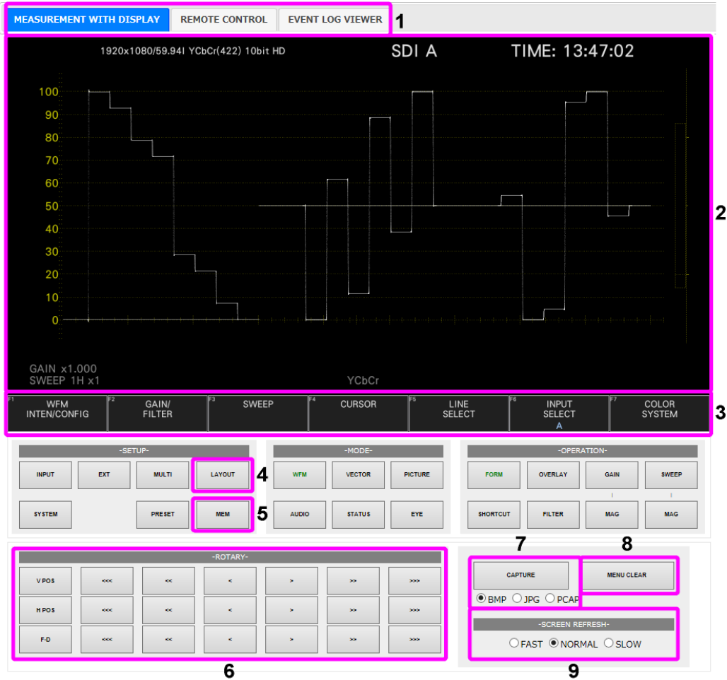
Figure 20-7 MEASUREMENT WITH DISPLAY
