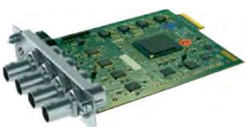
PHRXM-4AES Audio I/O 75 Ohm unbalanced
