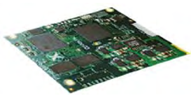
PHRXM-DOLBY Dual Dolby decoder Dolby E/D/Plus (mounted on CPU card)
