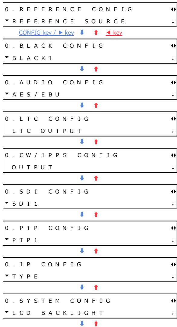
Except for some cases, a number is displayed at the upper left of the CONFIG menu. This number indicates the menu level. The larger the number, the deeper the level.
