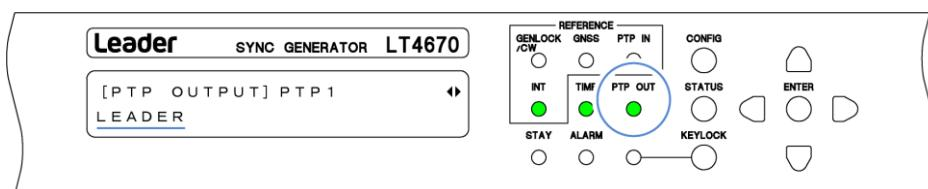
Note that when the BMCA function causes this instrument to enter the passive state, PTP OUT on the front panel lights in orange and the message changes to "PASSIVE".
