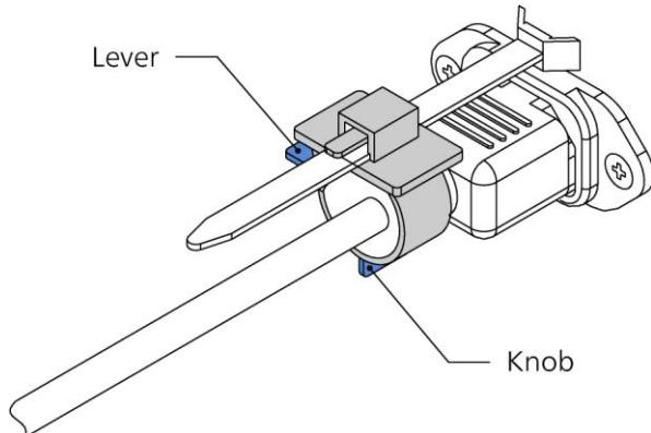
Figure 5-6 | Mounting the AC cord clamp 3
