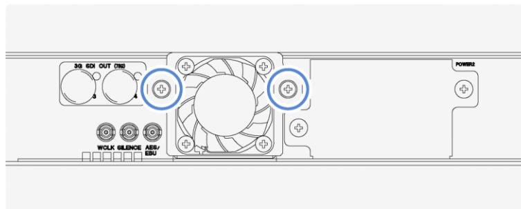
**4 Pull out the fan unit.**
