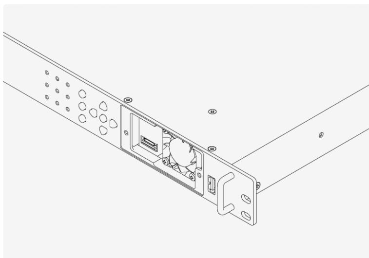
**6 Attach the fan cover, and tighten the two screws.**
