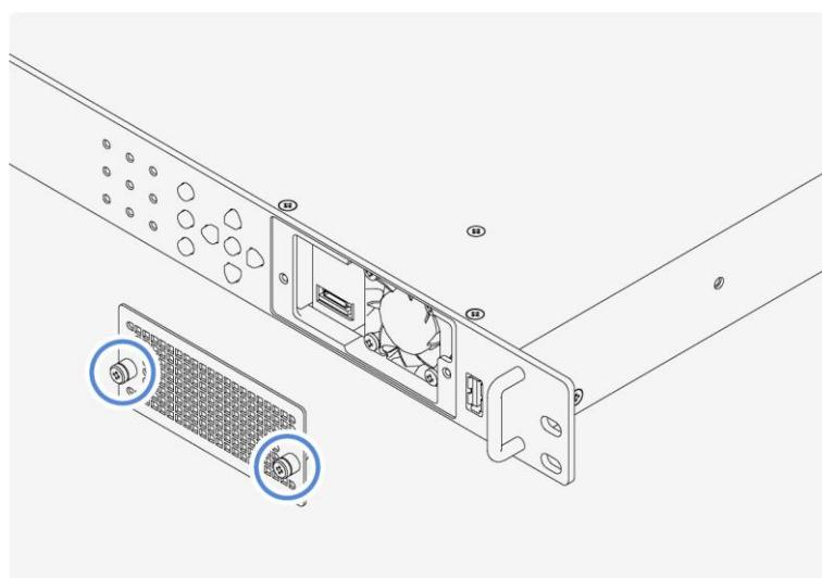
**4 Loosen the two screws on the front panel, and pull out the fan unit.**
