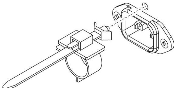
Figure 5-4 | Mounting the AC cord clamp 1
