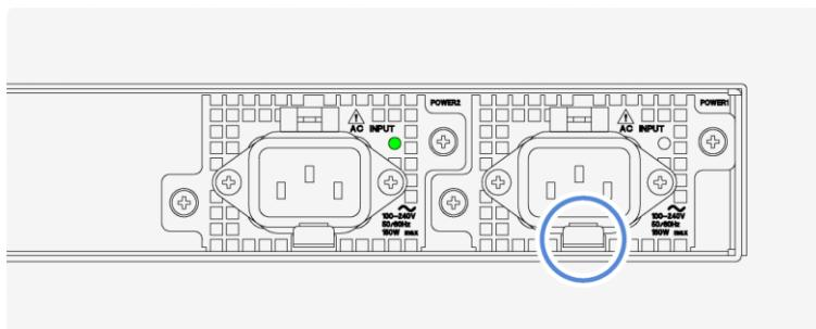
Next, with the lever pulled up, pull out the power supply unit.
