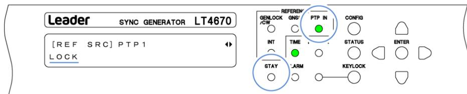
When REFERENCE SOURCE is set to PTP1/2, the PTP IN LED on the front panel is displayed as shown below according to the combination of the PTP1 state and the PTP2 state.
