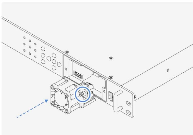
**5 Insert a new fan unit, and tighten the two screws.**
