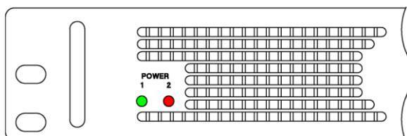
Figure 5-11 | POWER LEDs (when an error occurs)
