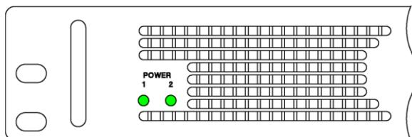
Figure 5-10 | POWER LEDs (during normal operation)
