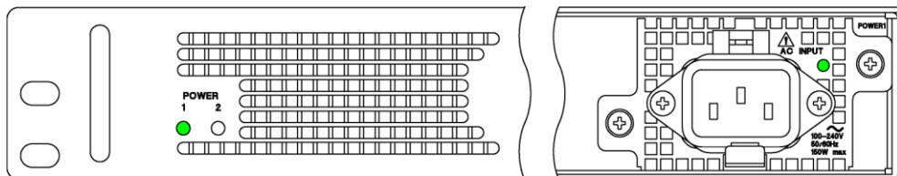
Figure 5-3 | POWER LEDs
