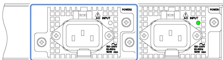
Figure 5-7 | Adding the power supply unit 1
