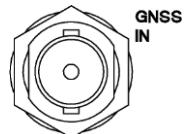
When you apply the signal, an "\*" is attached after "GNSS". In addition, the message changes to "ADJUST FREQ TO GNSS" > "ADJUST PHASE TO GNSS" > "TRACKING" in this order, and the reference signal is introduced. Wait in this state.
