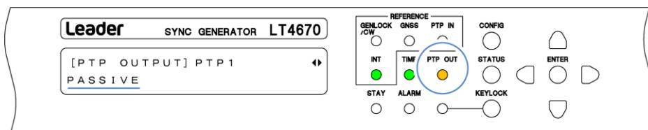
When PTP1 and PTP2 are both leaders, the PTP OUT LED on the front panel is displayed as shown below according to the combination of the PTP1 state and the PTP2 state.
