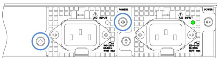
Figure 5-8 | Adding the power supply unit 2
