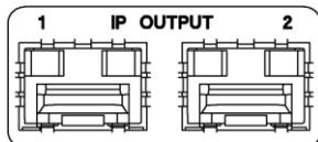
For IP signals, the patterns specified on the SDI CONFIG menu are output as follows. Up to four streams can be output per port within the band.
