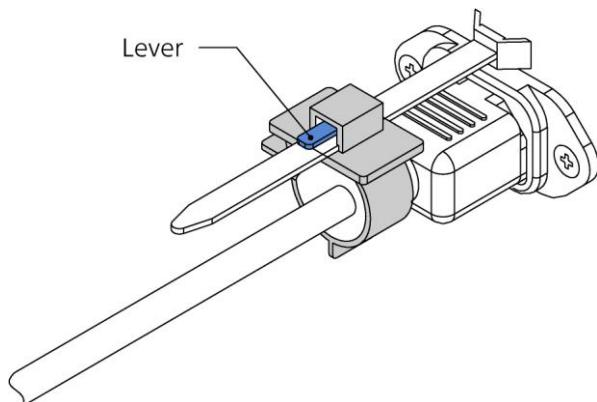
Figure 5-5 | Mounting the AC cord clamp 2
