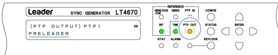
When the PTP output becomes normal, PTP OUT on the front panel lights in green, and the message changes to "LEADER". Use the instrument in this state.
