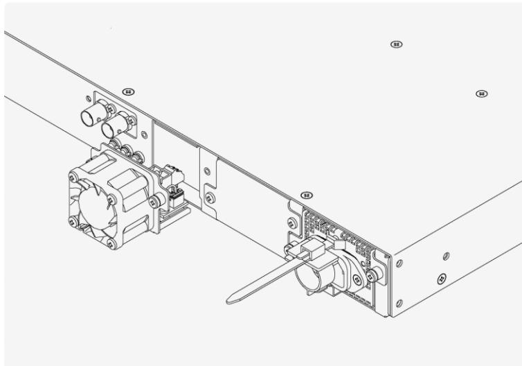
**5 Insert a new fan unit, and tighten the two screws.**
