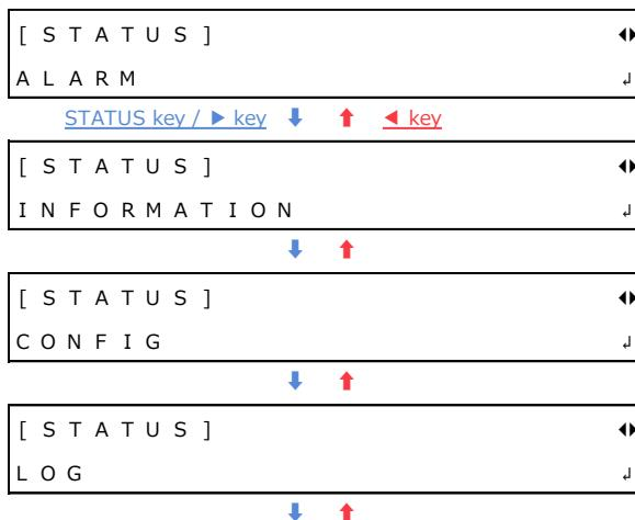
No levels are indicated on the STATUS menu. As with the CONFIG menu, to enter a lower level menu, press the ENTER key. To return to a higher level menu, press the STATUS key. When you are at a level other than the top level, hold down the STATUS key to return to the top level.
