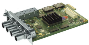
PHRXM-A Dual input 3G/HD/SD SDI single analyzer
