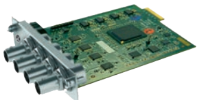
PHRXM-4 AES Audio I/O 75 Ohm unbalanced
