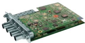
PHRXM-AGE Single input 3G/HD/SD SDI single analyzer with eye and jitter plus SDI generator
