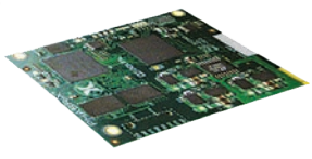
PHRXM-DOLBY Dual Dolby decoder Dolby E/D/D Plus (mounted on CPU card)
